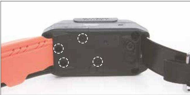
Open the antenna enclosure by removing the 4 screws and the contact points. Remove the screw holding the antenna in place to replace the antenna.
