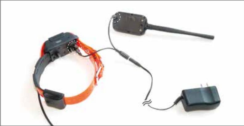
Fully charge the PATHFINDER GPS connector and GPS receiver before the first use. The PATHFINDER uses lithium polymer batteries.
