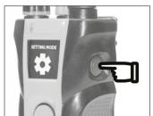
Make sure the transmitter is off. Hold the on/off button on the transmitter until there is a rapid green LED light on the transmitter and the OLED screen shows "Setting Mode \*"
