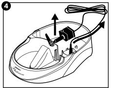
4. Remove the pump from the square indentation and pull the in-line plug up through the hole.
