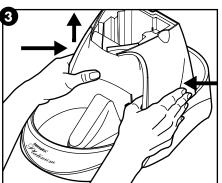
Remove the housing by pushing in on both sides and lifting up.
