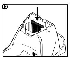
Rinse the carbon filter and insert it into the housing. It fits narrow side down, and the black side faces the front.
