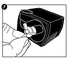
7. Use a fingernail to pull out the impeller, which is held in place magnetically.
