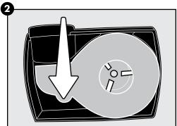
Use a fingernail to pull out the impeller, which is held in place magnetically. Clean the pump parts with warm water and soap. Reassemble the pump by first inserting the impeller. Then, replace the stator and faceplate.
