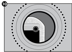
11. Insert the filter housing into the cone opening and push straight down. By pushing the filter housing all the way down to the rubber gasket, the filter housing should easily attach to the intake tube.
