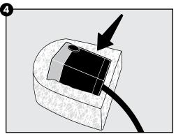
Place the assembled pump and foam filter inside the square indentation in the bowl. Position it so the circular opening on top of the pump is in the center of the bowl. Press down to engage suction cups.
